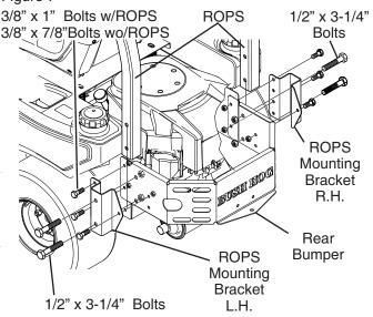
**B.** Attach the right hand and left hand frame brackets and the optional ROPS mounting brackets to the outside of the ZT frame as shown in (Figure 8). Use four  $3/8" \times 3/4"$  bolts or (six  $3/8" \times 1"$  bolts if ROPS is attached) and 3/8" locknuts.Tighten all fasteners, If ROPS is attached leave all fasteners slightly lose and proceede to next step.
